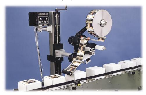
Weber's Alpha 86 combines speed with precision to create a line of widely versatile pre-printed label applicators. Pressure-sensitive labels are applied in-line using the reliable wipe-on method, where a label automatically is peeled from its liner, and then gently but firmly is affixed to the carton or product.
